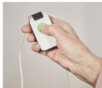
Emergency Call via Call Button 3 help calls (family, friends, neighbour) 1 emergency call (professional help, Call Center)
