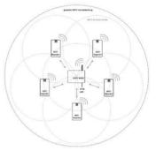
After registration place the Repeaters at their individual operational place and assure that the DECT Link quality (LED2 green) of each Repeater with respect to the Base station.
