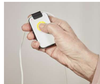
„easy subscription“ via Call Button Registration to home-based DECT station eg Fritzbox, Speedport, Gigaset, Panasonic, Philips
