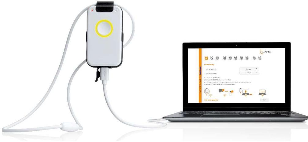
The driver of the PC APP can run only on computers with operating systems WIN7 or WIN10. You will find the driver installer and the PC App on the enclosed USB stick.
